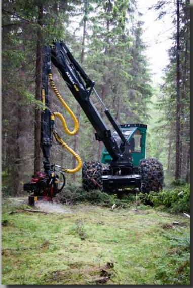
New dual circuit hydraulics allow more power for simultaneous use of crane and harvester head
