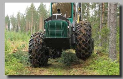
Optional hydraulic rear axle with automatic stabilization.
