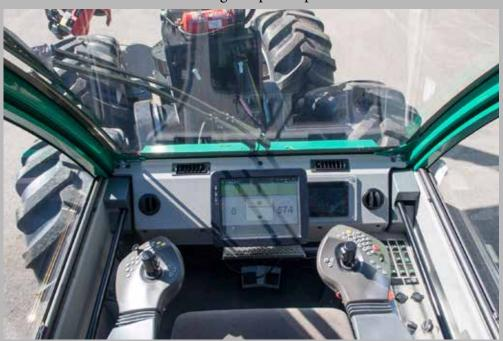
The basemachine operations are controlled with a highly customizable, flexible and operator friendly latest generation Iqan control system.
