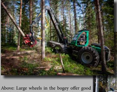
weight distribution even when working with maximum reach of the crane.
